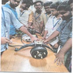
Front Axle Assembly With Suspension And Stub, Hub
