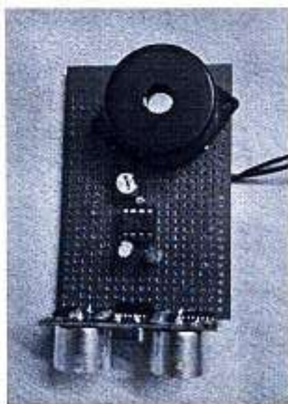
Fig 4.1: Ultrasonic sensor HC-SR04 interfaced with the Raspberry Pi
