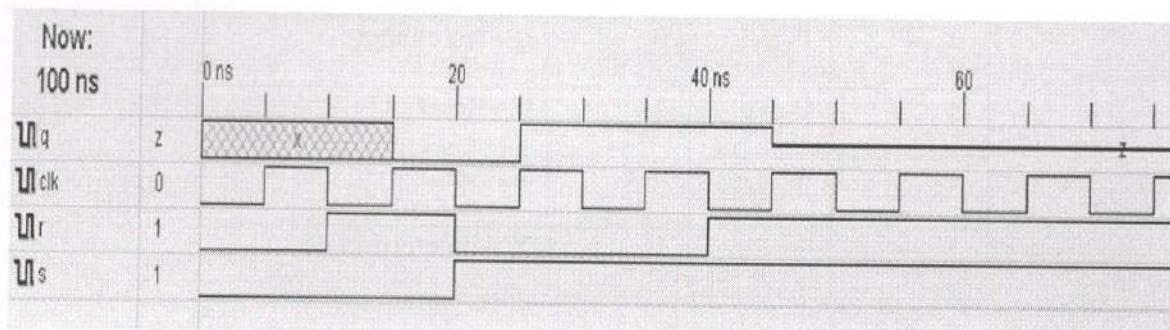
Testbench Output for T Flip Flop
