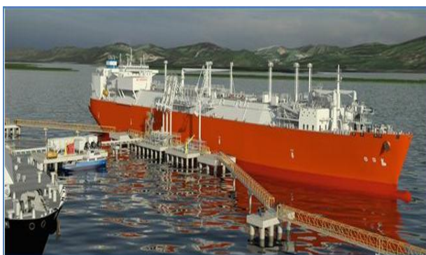
Fig. 3 Floating storage and Regasification unit (source: Aguirre Offshore GasPort)
